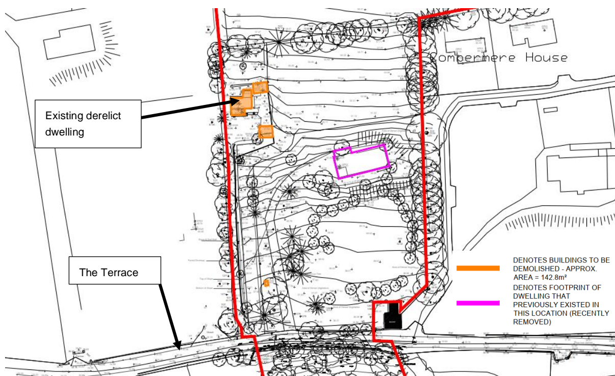
Figure 5 – Location of existing dwellings to be demolished
